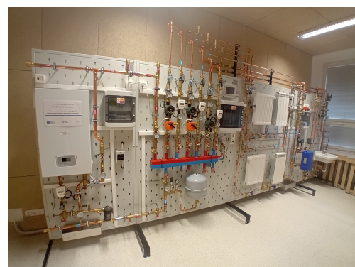
Fig. 2: Teaching interactive model – Building services measurement wall (Source: photo by author)
