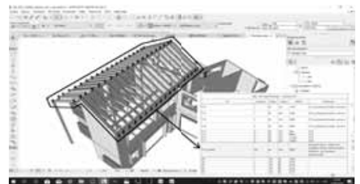
Picture 2.: List of elements generated from 3D model and its control (Source: M. Pavlas)
