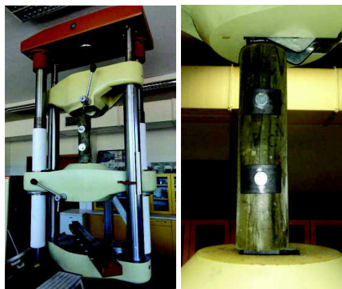
Fig. 9 Laboratory press (left), a sample with modified washers in the press (right).
