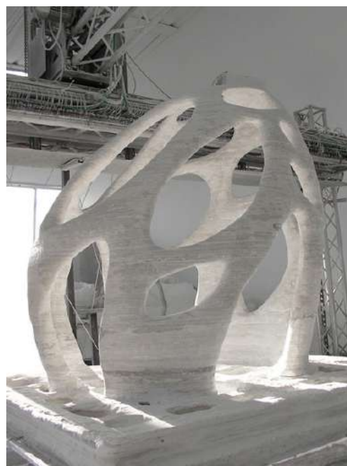
Fig. 3.: Radiolaria pavilion using D - Shape technology. (Source: Shiro, studio, 2009. Radiolaria pavilion by Shiro Studio. Dezeen. Available at: https://www.dezeen.com/2009/06/22/radiolaria-pavilion-by-shiro-studio/ [Accessed June 30, 2023])
