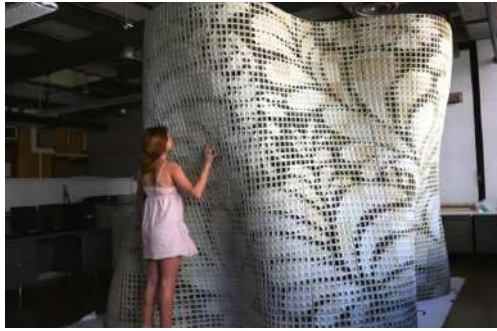
Fig. 4.: Pioneering research at UC Berkeley using powder-based material. (Source: Williams, A., 2015. Berkeley researchers pioneer new powder-based concrete 3D printing technique. New atlas. Available at: https://newatlas.com/berkeley-researchers-pioneer-powder-based-concrete-3d-printing/36515/ [Accessed June 30, 2023])
