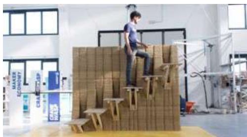
Fig. 12.: Prototype of a 3D printed earth wall. (Source: 3D Wasp, 2022. 3D printed earth wall with embedded staircase. 3D Wasp. Available at: https://www.3dwasp.com/en/3d-printed-wall/ [Accessed June 30, 2023])
