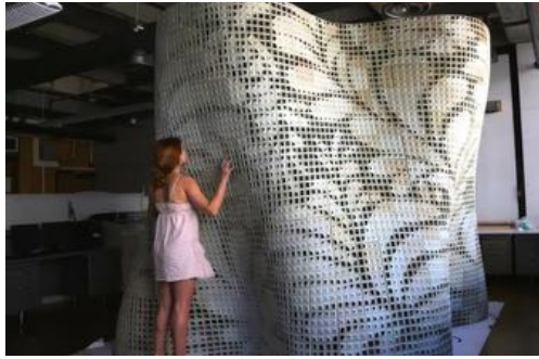
Fig. 4.: Pioneering research at UC Berkley using powder-based material. (Source: Williams, A., 2015. Berkeley researchers pioneer new powder-based concrete 3D printing technique. New atlas. Available at: https://newatlas.com/berkeley-researchers-pioneer-powder-based-concrete-3d-printing/36515/ [Accessed June 30, 2023])
