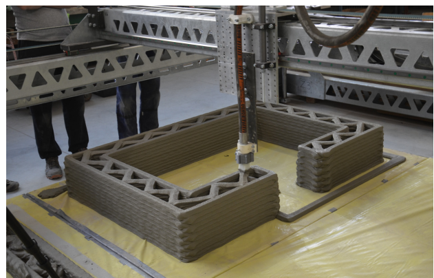
Fig. 1: Example of printed wall segment
