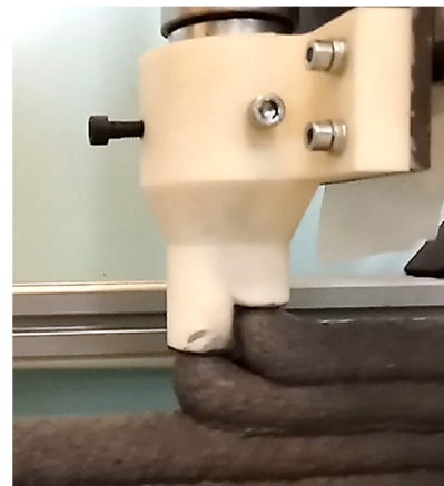
Fig. 1: Concept of printing with using dual-exit nozzle.
