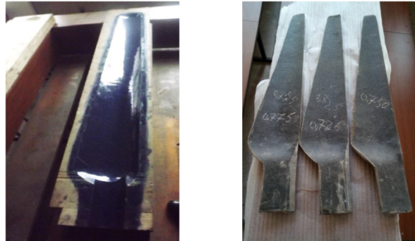
Fig. 2: Basalt composite blade products blade mold-shape (left); Basalt composite blade products blade mold-shape L=700\text{mm} , B=150\text{mm} , b=35\text{mm} (right).
