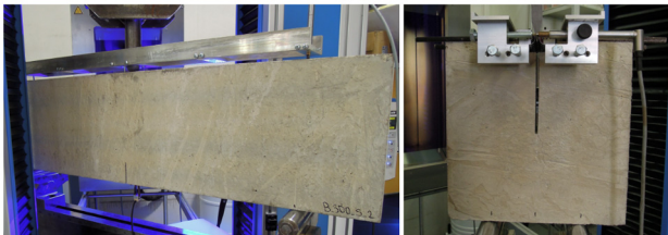
Fig. 1: Test configurations of a three-point bending test (left) and wedge-splitting test (right).
