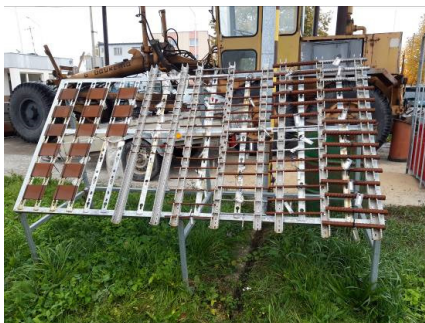
Fig. 1: Measurements of corrosion losses – measurement station (exposure) in the town of Martin, Slovakia.
