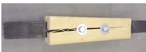
Fig. 1: A specimen of a squared timber connection after failure.
