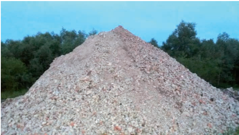
II.2. Recycling aggregate from concrete and brick, photo Mohamed Ahmad. 16.06.2016
