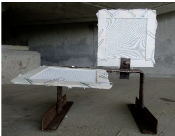
Figure 12: The method of “dry plates” for the determination of chloride deposition (horizontal and vertical position)
