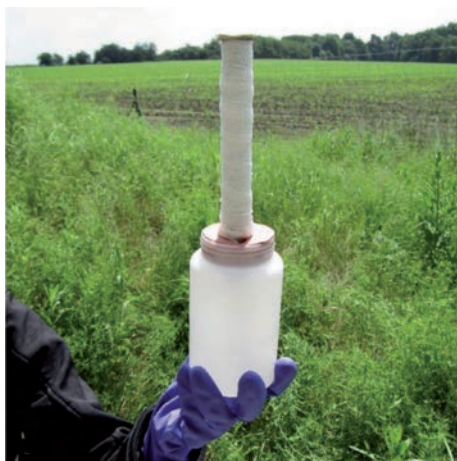
Figure 11: "Wet candle" method for the determination of chloride deposition
