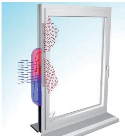
II. 3 Ventilation in the i-Tec Smart Window [12]
