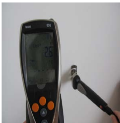
II.3. The humidity of the wall and the heat transfer coefficient for a warmed wall were measured using Multifunction Testo 435-2.
