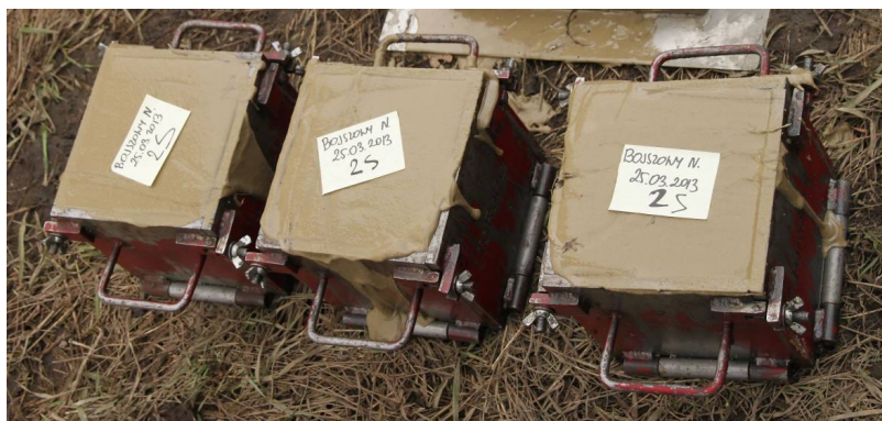
Fig.4: Samples of cement grout material taken from columns during injection process (own photo)
